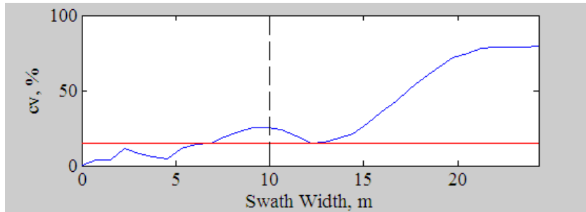
Figure 13. CV versus Swath width plot showing a CV of 27% at a swath width of 10 m.
