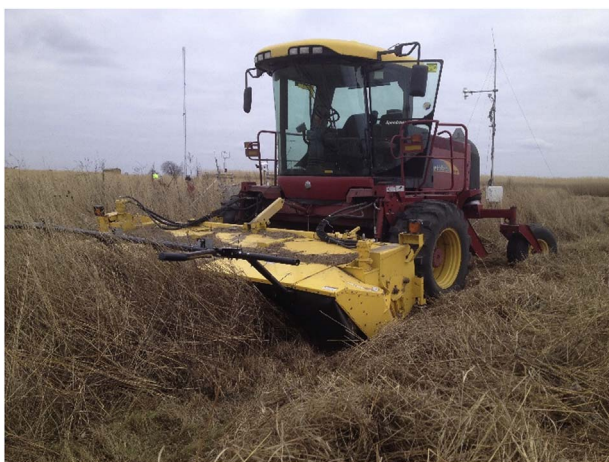
Fig. 1. New Holland H8080 self-propelled mower-conditioner with 750 HD specialty rotary disc head.
