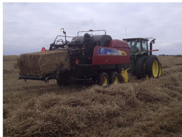
Fig. 2. New Holland BB9080 large square baler powered by a John Deere 7930 tractor.
