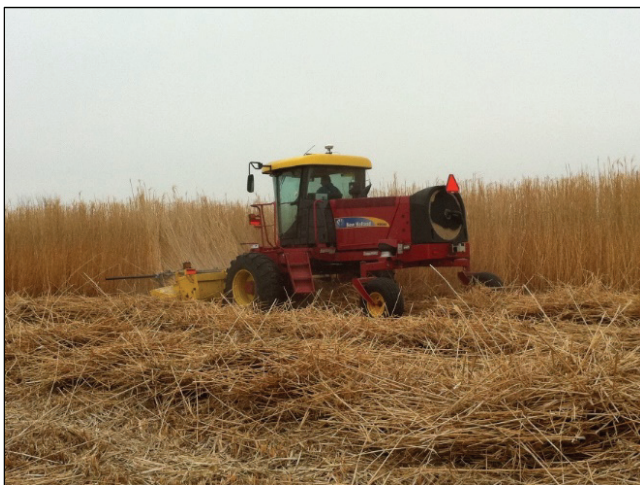
Figure 2. New Holland H8080 self-propelled mower-conditioner with 750 HD Specialty rotary disc head.
