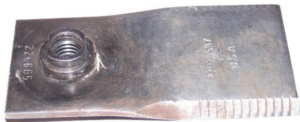
Figure 1. Blade typical of those available for use on a rotary mower (New Holland part no. 87029587).
