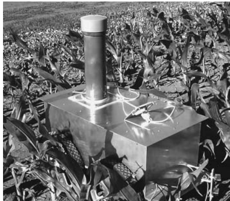
AgTracker, a rugged, simple, and inexpensive robot for scouting applications.
