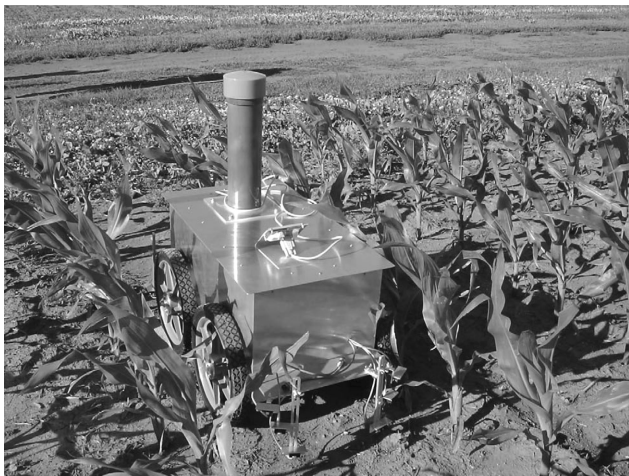
Fig. 2 AgTracker, a simple, low-cost crop-guided Agricultural Robot.
